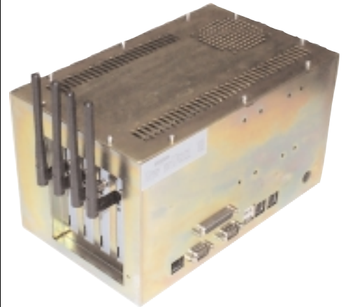
Shown in the picture is our solution Wireless Access Point IEEE802.11b customized with a 44Mbit/s using the Board MODO and Optional case.
